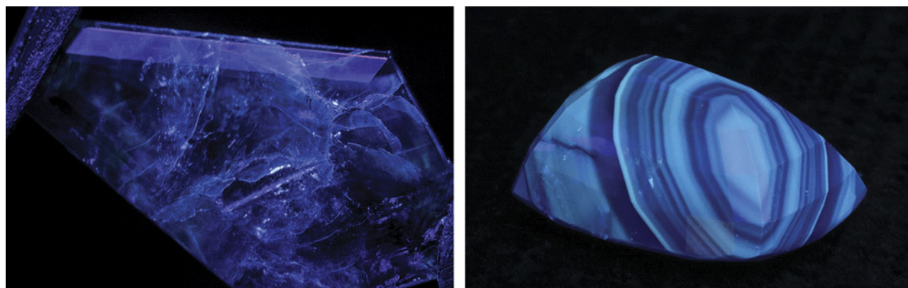
Figure 7. Left: An emerald seen in long-wave UV, highlighting the filled fractures in the stone. Photomicrograph by Nicole Ahline; field of view 19.27 mm. Right: A heated natural blue sapphire emits chalky blue to green fluorescence in short-wave UV. Photo by Nicole Ahline and Jessa Rizzo.
