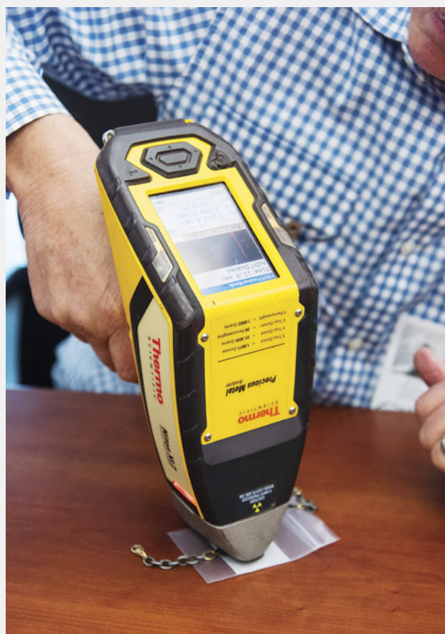
Figure A-2. The Thermo Scientific Niton XL2 is the portable XRF device used by GIA to quickly test precious metals. Photo by Emily Lane; courtesy of Hallock Coin.
