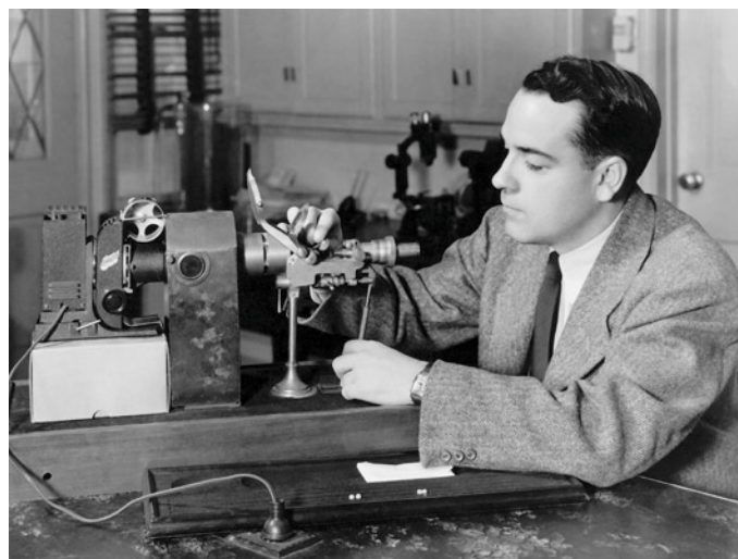
Figure 10. Left: Richard Liddicoat using an endoscope to examine the internal structure of a pearl. Right: A 1979 photo of the same instrument.
