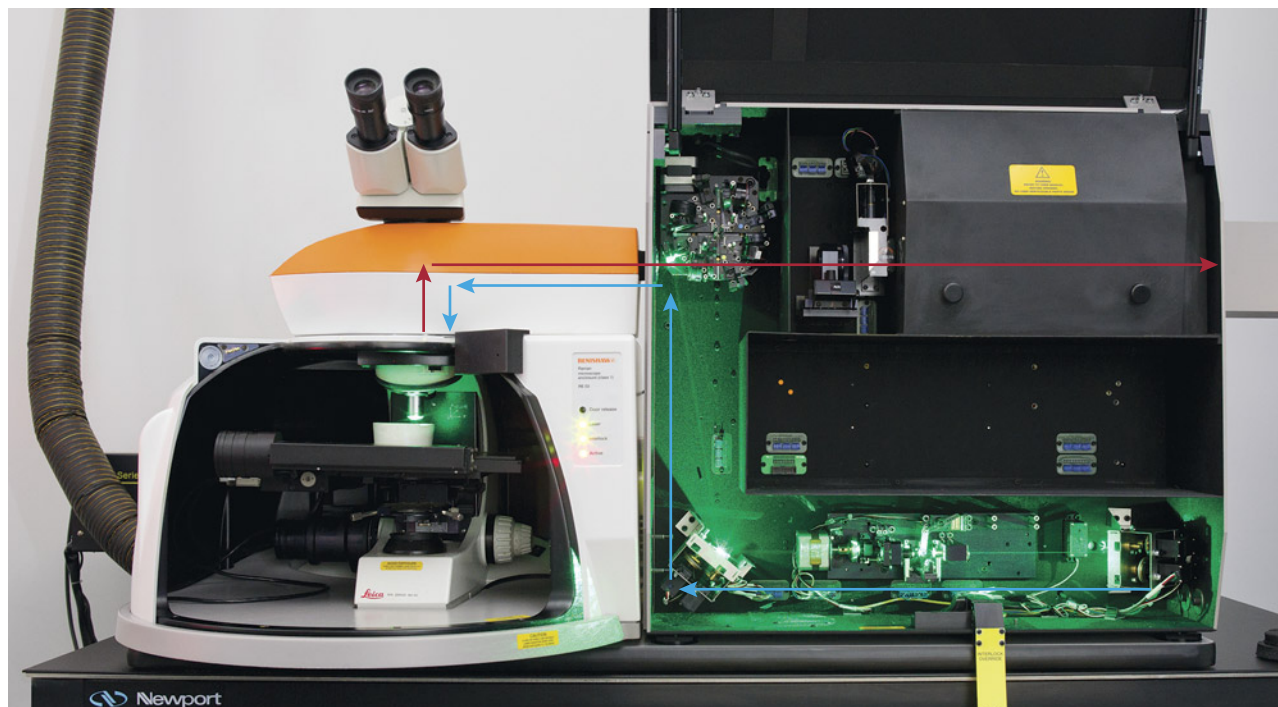
Figure 6. The Renishaw inVia confocal Raman microscope is a popular research-grade Raman spectrometer. Samples are placed on the microscope stage under the objective lens for analysis. The protective doors are open here to show the internal path of the laser beam. The green light is scattered light along the optical path of the 514.5 nm argon laser, which is mounted behind the instrument. Photo by Kevin Schumacher.
