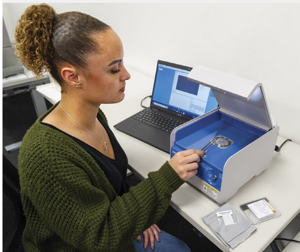
Figure A-1. The Horiba Mesa-50 XRF is used by GIA's laboratories. Gemstones and jewelry pieces can be placed on top of the testing window. A laptop is connected to the testing unit, and the system also has a built-in camera that allows the user to adjust the position of the X-ray beam on the sample. Photo by Kevin Schumacher.
