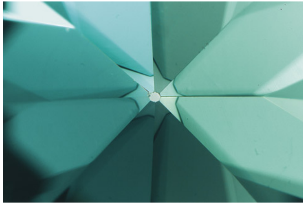
Figure 5. This “umbrella effect” at the culet of a diamond was created by cyclotron treatment, a type of artificial irradiation. Photomicrograph by Nicole Ahline; field of view 2.90 mm.
