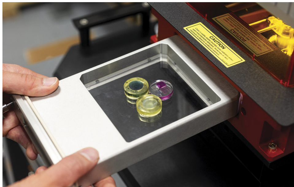
Figure 4. LA-ICP-MS analyses are standardized with NIST glass standard reference material (the blue and colorless pieces in yellow epoxy) for a variety of elements. Also shown is our internally developed matrix-matched corundum standard (colorless epoxy with four variously colored sapphires) used specifically for ruby and sapphire analysis. Photo by Kevin Schumacher.
