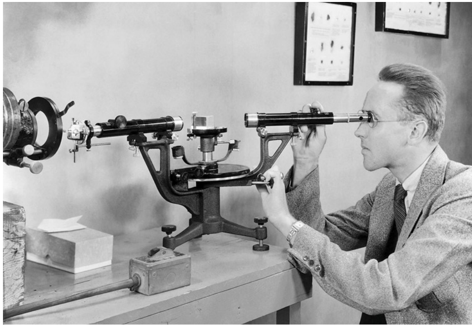
Figure 8. Robert Shipley Jr. using a spectroscope to examine the absorption spectrum of a gemstone at GIA for a 1937 Paramount Pictures film for its “Popular Science” series.
