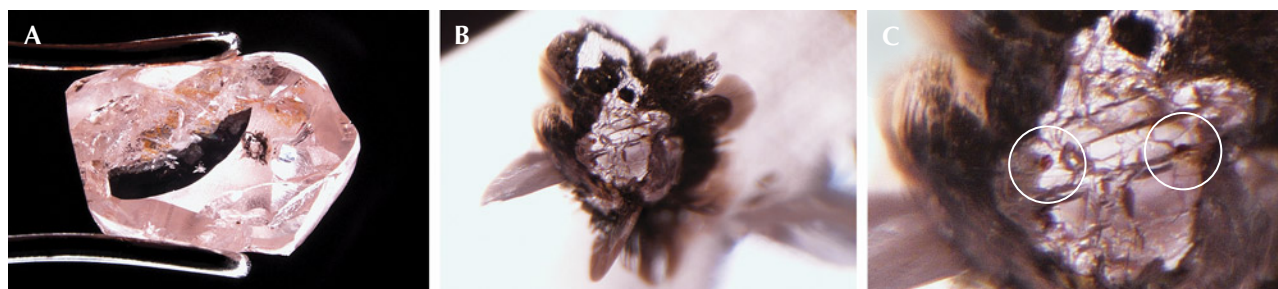
Figure 3. An inclusion-bearing pink superdeep diamond. The largest inclusion is a two-phase mixture dominated by colorless breyite ( \text{CaSiO}_3 ) and small spots of brown perovskite ( \text{CaTiO}_3 ), the latter circled in image C. The inclusion is surrounded by graphitized fractures that appear black. The original rough weight was 1.37 ct, before windows were polished to examine the inclusions. Photomicrographs by Evan M. Smith; fields of view 14.52 mm (A), 1.42 mm (B), and 0.50 mm (C).
