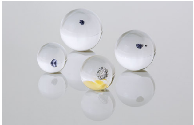
Figure 14. Weighing between 3.07 and 10.53 ct, these four small transparent colorless spheres of rock crystal quartz each hosted an opaque black inclusion (one sphere contained two inclusions). Photo by Annie Haynes.
