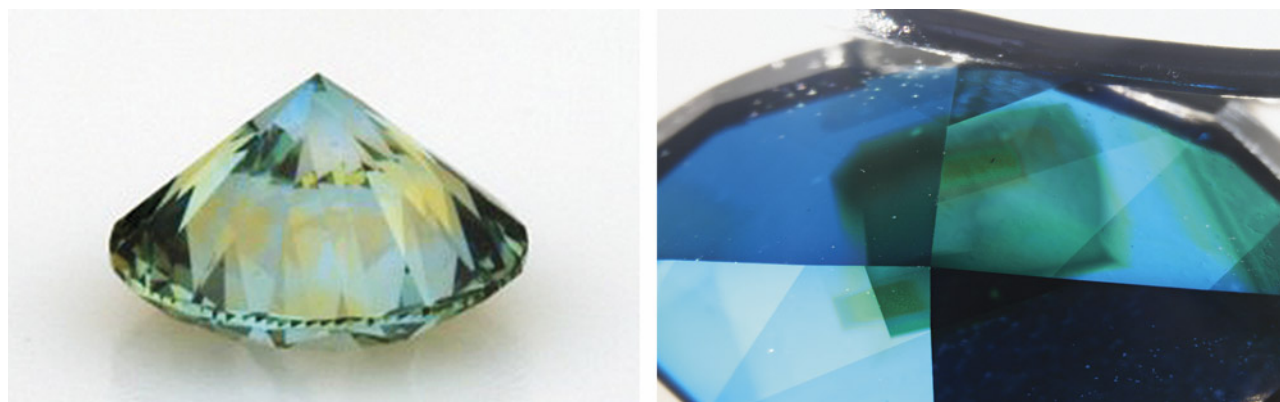
Figure 7. Viewed through the pavilion, sector-dependent color zones were apparent in both the round brilliant (left) and the marquise (right; field of view 7.19 mm).
