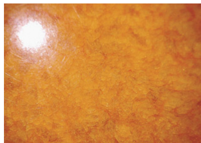
Figure 12. The 140.58 ct sphere exhibited a mosaic structure, and orange color concentration was noted within areas under magnification. Field of view 6.92 mm.
