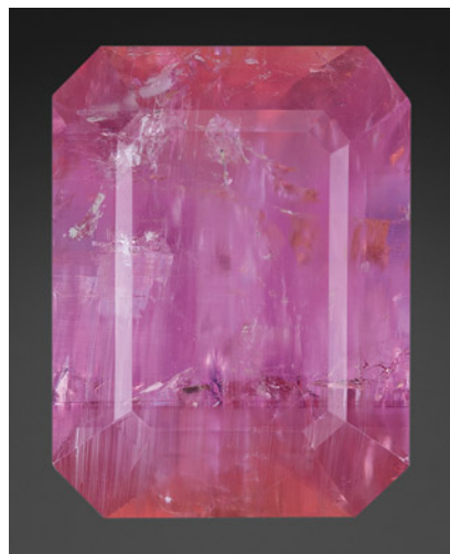
Figure 24. This 8.13 ct pezzottaite contains delicate growth banding (~horizontal) and tube inclusions (~vertical, seen best in lower left).
