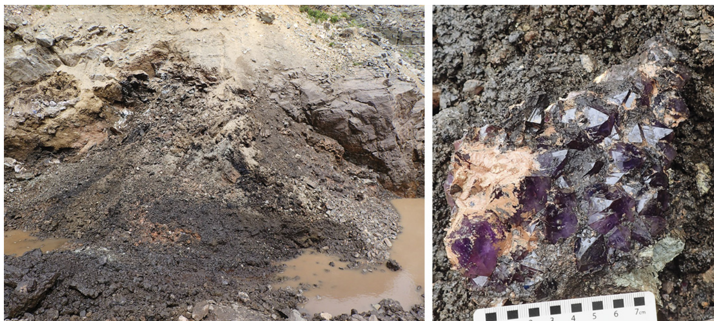
Figure 3. Left: The trench face in the main zone (in 2021) showing amethyst-bearing black mud in front of the vein's hanging wall. Right: Freshly recovered amethyst cluster in black and tan mud. Many clusters are completely obscured by the thick black to brown clay. Photos by Philippe Belley.
