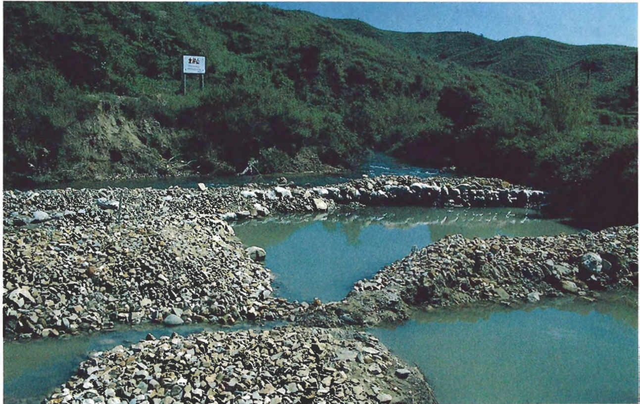
Figure 3. Various sections of this small portion of Ginxi Stream have been dammed up so that the miners can retrieve the gem gravel from the drained stream bottom.
