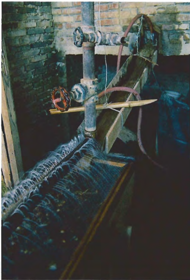
Figure 4. In the first of a five-step recovery process, the smaller gravels are passed through a 2.5-cm mesh; the larger material that remains on top is removed by hand.
