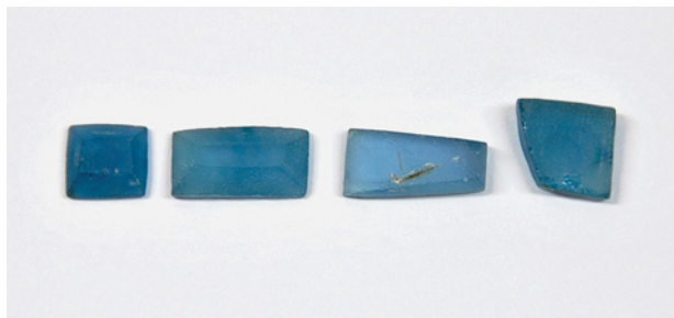
Figure 4. These four samples (9.5–16.5 mm long) had residual radioactivity higher than the exemption level when initially measured after 95 days. From left to right: Topaz-8, Topaz-9, Topaz-10, and Topaz-15. Photo by J. Zhang.
