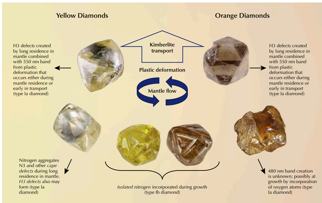
Figure 8. Some color centers are created during diamond growth in the mantle, while others are acquired after long residence times at high temperatures or during plastic deformation that might occur due to mantle flow or during initial stages of transport in kimberlite.
