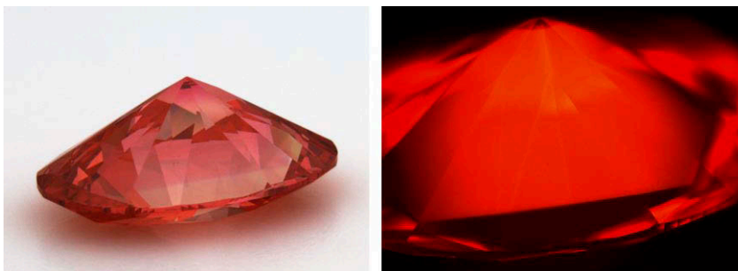
Figure 24. Left: Strong color zoning observed under natural lighting conditions. Right: The fluorescence pattern follows this zoning, as observed in the DiamondView image (strong short-wave UV).
