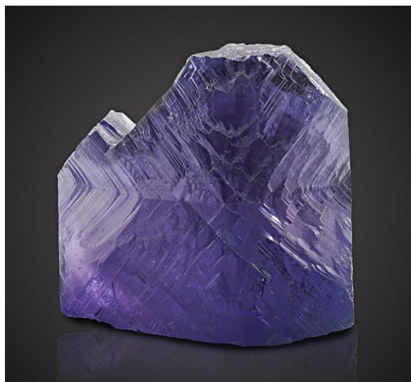
Figure 11. The pronounced pleochroism of the rough spodumene crystal weighing 2,950 grams, seen here in two orientations, was one of the properties that had to be considered during fashioning. Photos by Arjuna Irsutti.
