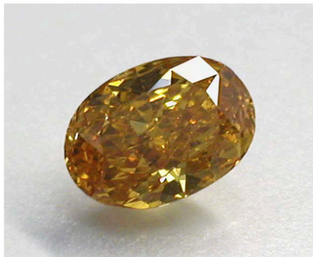
Figure 7. When gently heated, diamonds colored by a 480 nm band will temporarily change color to a more orangy hue. Photos by Wuyi Wang.
