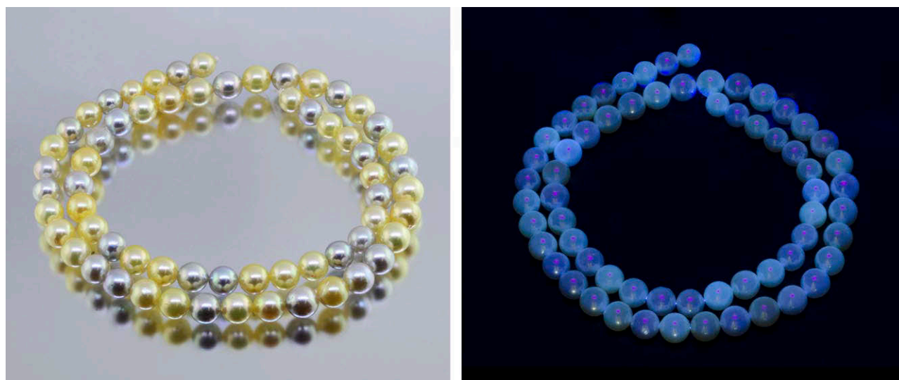
Figure 5. A strand of non-bleached and non-brightened akoya cultured pearls of various colors (left) and their varied fluorescence reactions under LWUV radiation (right). Photos by Sood Oil (Judy) Chia.
