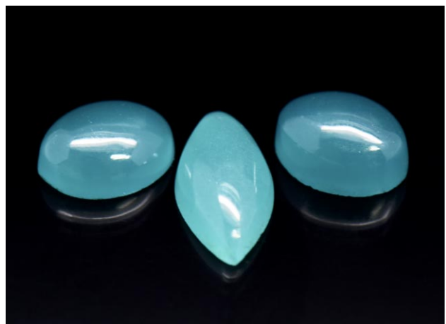
Figure 30. Two oval and one marquise cabochon of greenish blue glass samples ranging from 2.17 to 2.60 ct. Photo by Min Ye.
