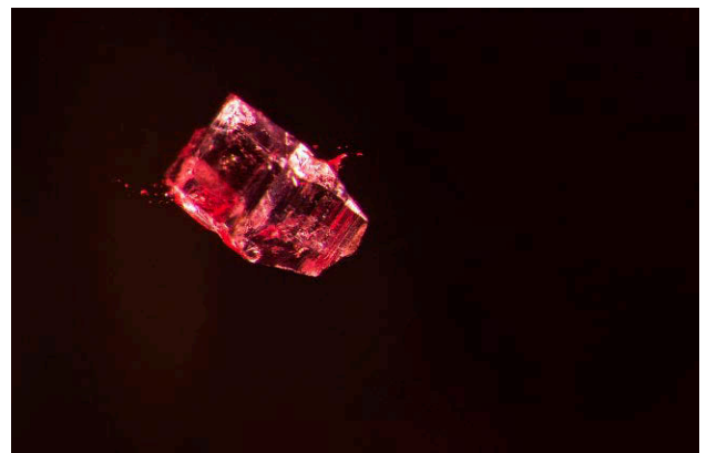
Figure 5. In darkfield illumination, cleavage was visible inside the crystal. Micro-Raman analysis showed it to be fluorophlogopite. Photomicrograph by Richard W. Hughes, darkfield illumination; field of view 2.5 mm.
