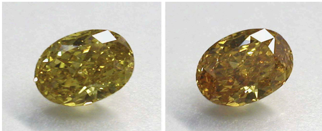
Figure 7. When gently heated, diamonds colored by a 480 nm band will temporarily change color to a more orangy hue. Photos by Wuyi Wang.
