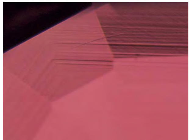
Figure 14. This 1.02 ct orangy red round brilliant exhibited hexagonal growth zoning when viewed down the c-axis. Photomicrograph by James Shigley; magnified 10 \times .
