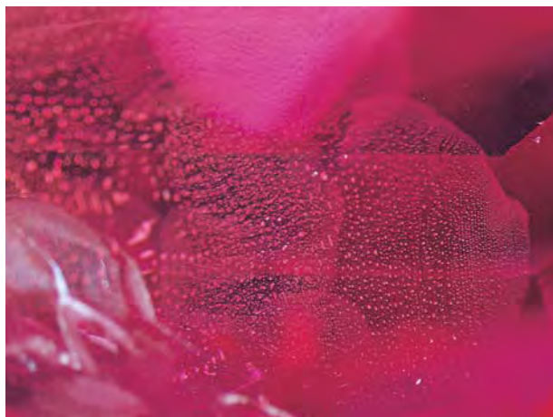
Figure 13. "Fingerprint" inclusions such as the one shown here are typical of red beryl. Photomicrograph by James Shigley; magnified 20 \times .
