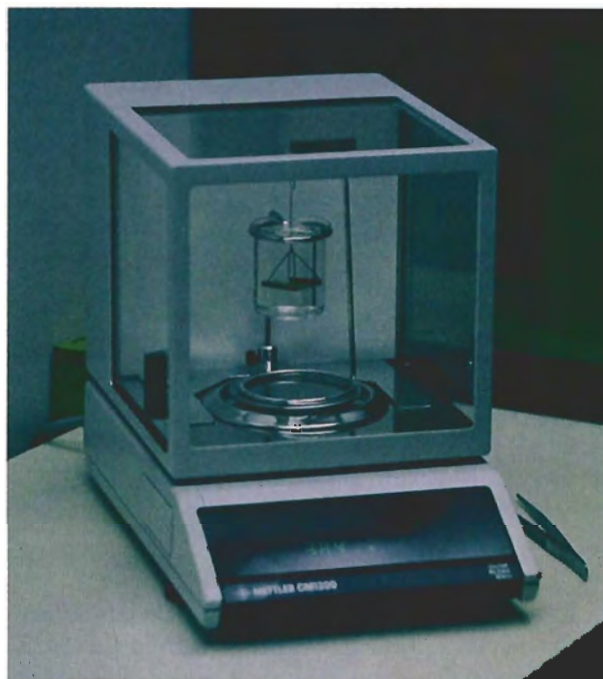
Figure 4. A Mettler balance with hydrostatic-weighing accessories was used to test the specific gravities of the karat-gold reference samples. Photo by Maha Smith-DeMaggio.
