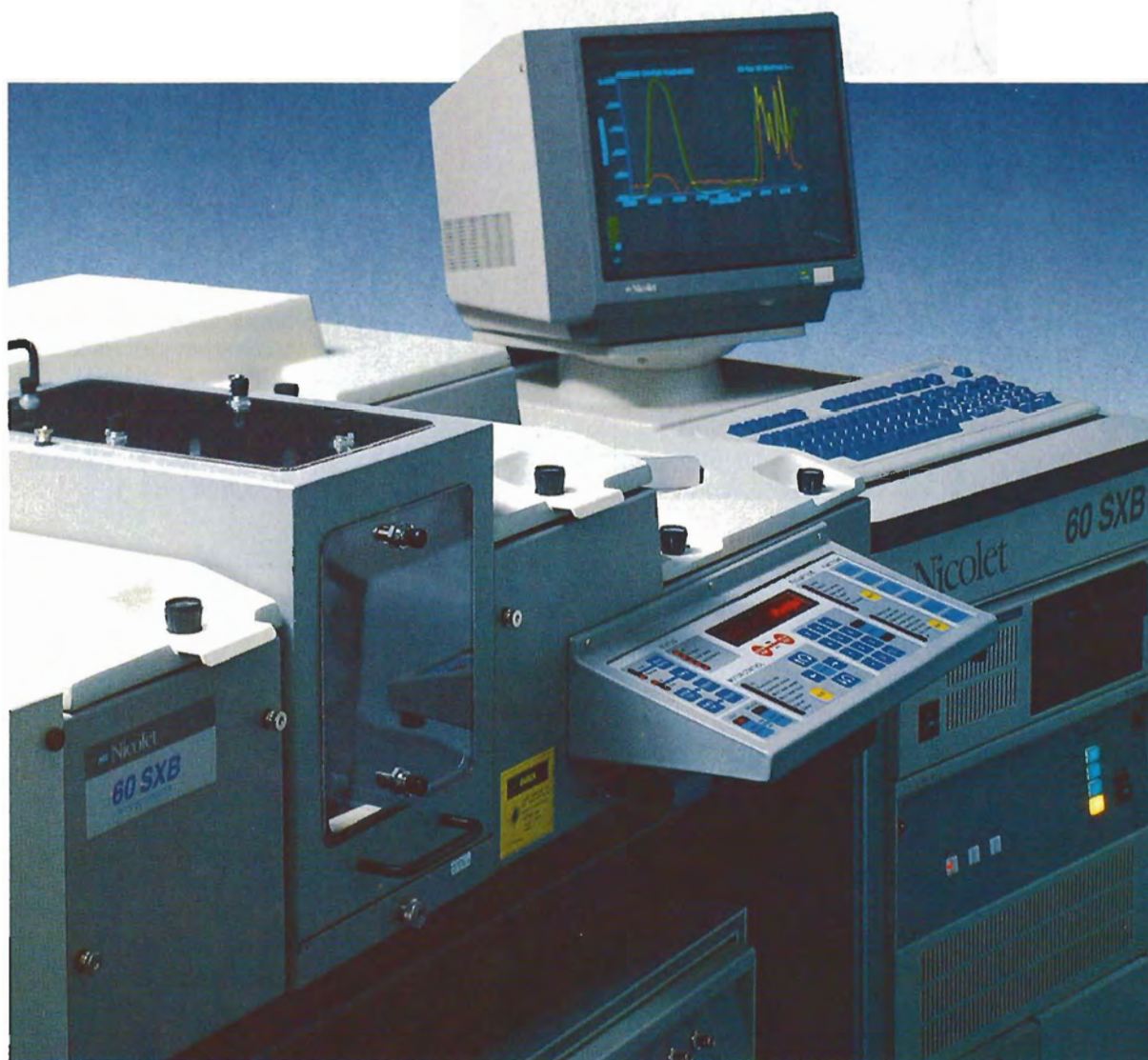
Figure 1A. The Nicolet 60SX FTIR spectrometer. Photo courtesy of Nicolet Instrument Corp.
