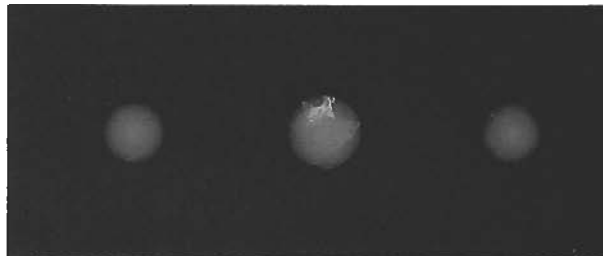
Figure 1. The white areas in this X-radiograph represent the filled cleavages and cracks in these three treated diamonds (the largest weighs 1.49 ct). X-radiograph by Tom Moses.
