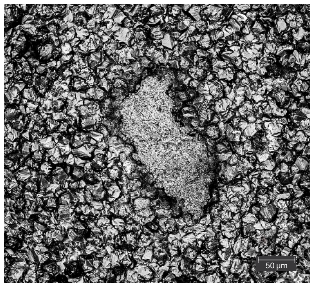
Figure 3. Photomicrography with a laser scanning confocal microscope system reveals an irregularly shaped impurity center within a brown spot. Image by Jian Zhang.
