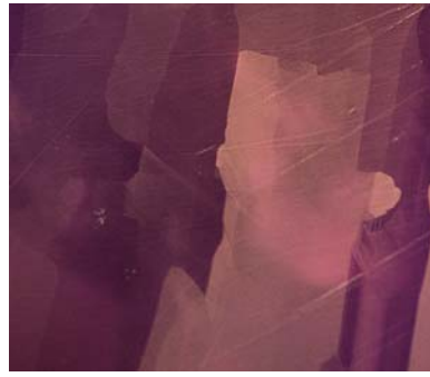
Figure 31. The subtle mosaic structure becomes visible when the synthetic sapphire block is rotated 90° from the optic-axis direction (left). As the microscope's analyzer is rotated, some of the blocks in the mosaic pattern become dark, while others appear lighter (right). Photomicrographs by John I. Koivula; magnified 10x.
