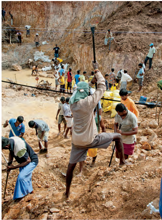
Figure 22. Sri Lankan miners work the sapphire deposit with hand tools. Photo by V. Pardieu.
