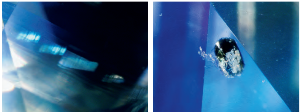
Figure 10. Parallel arrays of ribbon-like inclusions with jagged edges showed iridescence in certain directions (left, 45x). Dark green actinolite inclusions (right, 90x) were observed in one of the samples. Photomicrographs by K. S. Moe.
