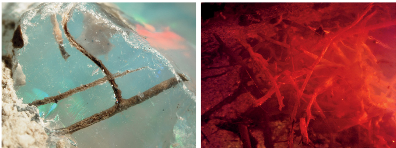
Figure 9. Irregular tube-like inclusions that appear to be fossilized plant matter occurred in both the Wollo opal (left, image width 4.4 mm) and the dyed opal (right, image width 5.0 mm) samples. Photomicrographs by S. F. McClure.
