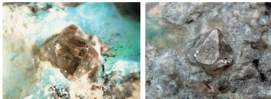
Figure 14. Well-formed quartz crystals with very short prism faces were visible in the matrix of both Wollo opal (left, image width 2.3 mm) and the dyed purple material (right, image width 1.4 mm). Photomicrographs by S. F. McClure.
