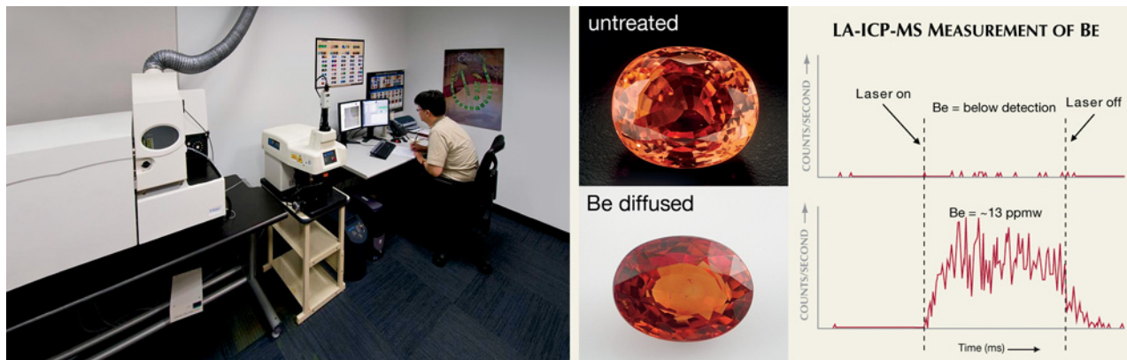
Figure 5. Beryllium-diffusion treatment of sapphire to produce padparadscha-like and other colors led to the widespread use of LA-ICP-MS in gem labs. The untreated stone is 88.11 ct and the Be-diffused sample is 2.16 ct. Photos by Kevin Schumacher (left) and Robert Weldon (center).
