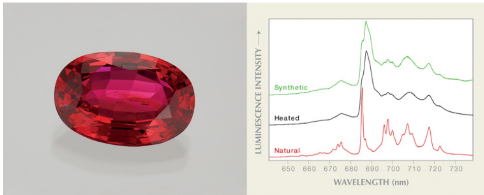
Figure 7. Photoluminescence analysis of red spinel (here, 10.42 ct) can separate natural from synthetic and heat-treated samples. Spectra are offset vertically for clarity. Photo by Robert Weldon.
