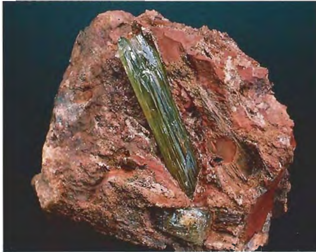
Figure 4. A 5-cm-long cigar-shaped crystal of yellowish green beryl is shown here in the massive reddish brown microcrystalline quartz (jasper) in which it was found at Luumäki. Photo by Jari Väättäinen.
