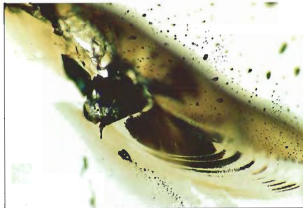
Figure 12. In this heat-treated yellow beryl from Luumäki, the once fluid-containing cavities are now empty. They appear dark because of total reflection of transmitted light. Note, too, the different appearance of the micro-fractures that surround the inclusion. Photomicrograph by Kari A. Kinnunen; magnified 32 \times .
