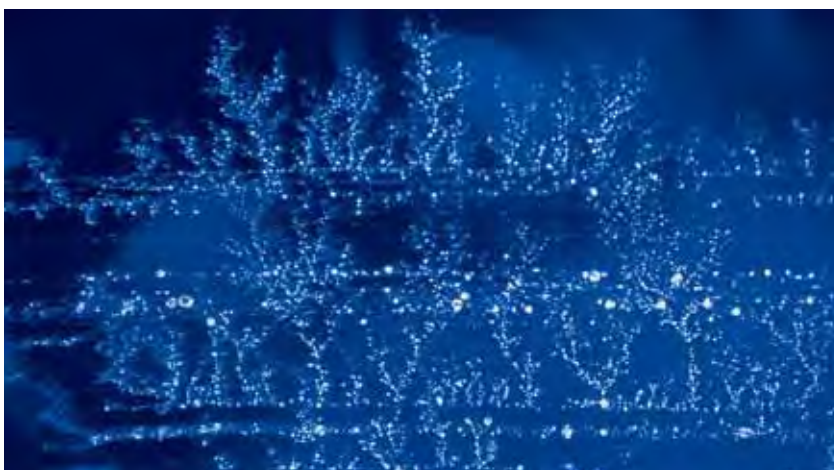
Figure 17. The rows of unusual tree-like inclusions in this sapphire probably formed through exsolution as a result of the heat-treatment process. Their composition is unknown. Magnified 10 \times .
