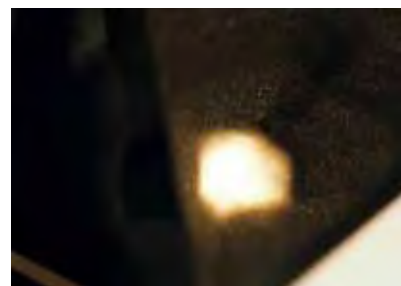
Figure 12. Unlike the cubic growth sectors, the black diamond’s octahedral sectors contained no micro-inclusions, and these areas consequently formed transparent “windows” through the stone. Magnified 45×.
