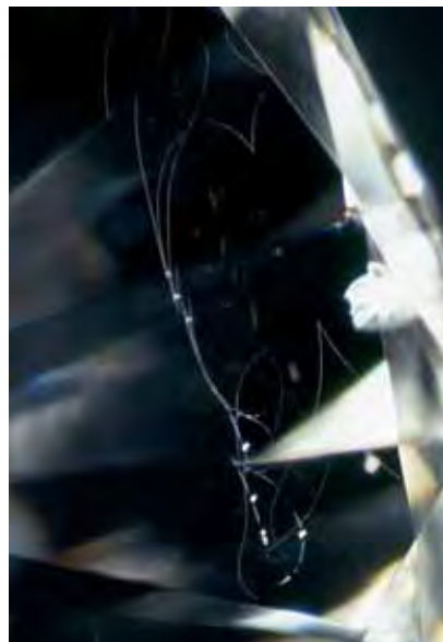
Figure 3. Microscopically visible filamentary “dislocation trails,” like the curved loops shown here, are very unusual internal features in diamond. Magnified 15 \times .
