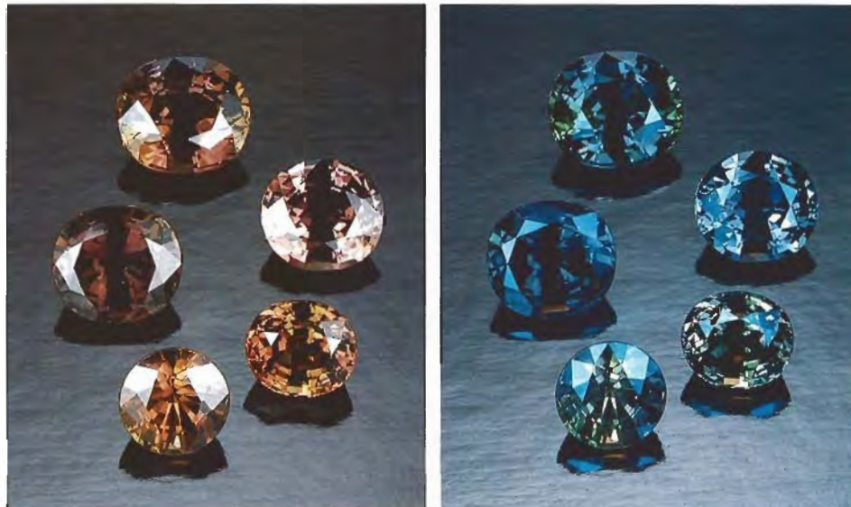
Figure 8. These five sapphires, ranging from 1.32 to 2.14 ct, show different colors in incandescent (left) and fluorescent (right) light. They are all reportedly from a new deposit in southern Tanzania. Courtesy of DW Enterprises; photo © GIA and Tino Hammid.
