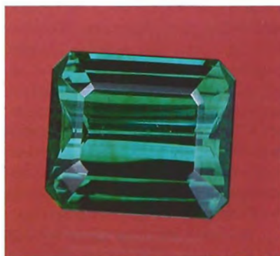
Figure 10. This 12.30-ct synthetic green quartz had been misrepresented to our client as a new type of natural quartz from Brazil.
