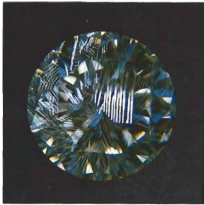
Figure 4. These long, blade-like inclusions produce a kaleidoscopic effect when this 0.75-ct. diamond is viewed faceup. Magnified 16 \times .
