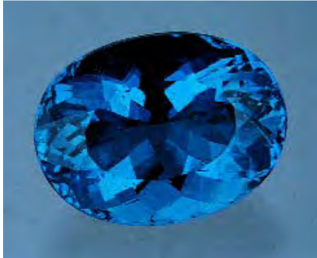
Figure 35. This 9.84 ct irradiated fluorite appears deep blue in daylight-equivalent fluorescent light (as shown here) and purple in incandescent light. Photo by Maha Tannous.
