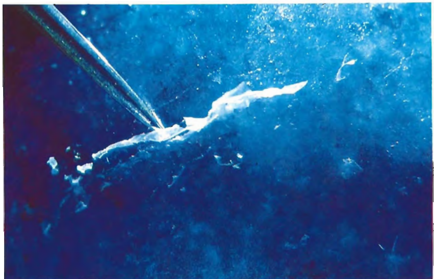
Figure 6. Brush probe reveals wax coating on treated lapis lazuli. Magnified 10x.
